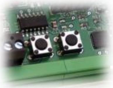
The Central-ANTC IDV32 doesn't need PC to be installed in the field, because once you set the current date and time stored and maintained by lithium backup battery (operation usually carried out prior to shipping), simply insert the key into the slot and, using the 2 buttons to the board, press to set the NORTH and then press to start and / or stop the running log. A practical green LED flashes to tell you if the log is written or not.
